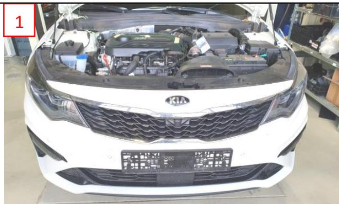
*Loosen the mounting screws and clips of the front bumper on the radiator support, fenders, underbody and the wheel housings. Remove the front bumper (1).*
